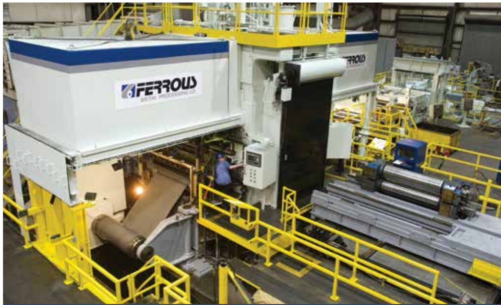
With 3,000 tons of rolling force, the four-high cold mill at Ferrous Metal Processing produces cold-rolled strip with a consistent gauge and shape on a toll basis. (Photo courtesy FMP)
