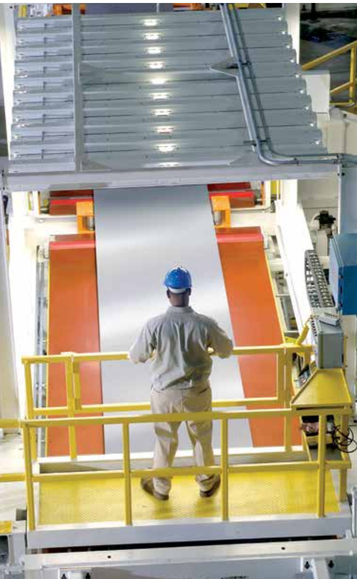
A worker at Ferrolux Metals, Wayne, Mich., inspects cold-rolled sheet destined for exposed automotive use. (Photo courtesy Ferrolux)
